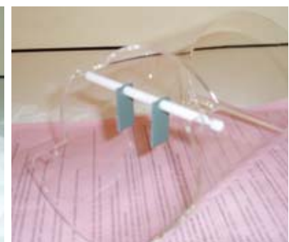
Haynes 230 alloy test sample, before (mirror finish, left), and after exposure to a 900 °C helium stream, in the presence of impurities, in the CORINTH facility for the investigation of impurities in helium, at CEA/Saclay. The test evidences uniform sample corrosion.
